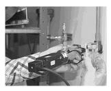
3 Attach the flow meter to the measurement chamber. The flow meter must be aligned in such a way that the scale has a vertical position.
