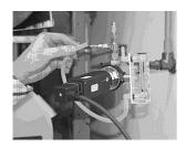
3 Now the hose connection from the hose nozzle of the precision measurement chamber is lead to the lower connection of the flow meter.
