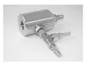
Through the precision measurement chamber, a defined incident flow of the sensor is enabled for all process pressure levels from 1 to 35 bar. Using a fine metering valve, it is possible to set the optimal sensor incident flow of 1 I/min for each different process pressure (1 - 35 bar).
